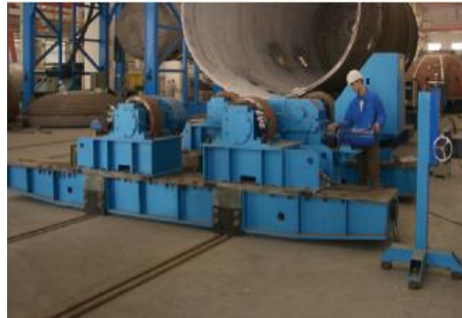
200 tons anti-drift welding rotators
