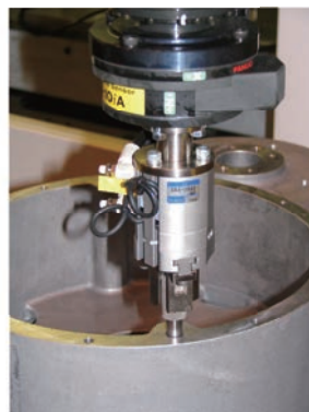
Dimension check of holes (Gage insertion by force control)
