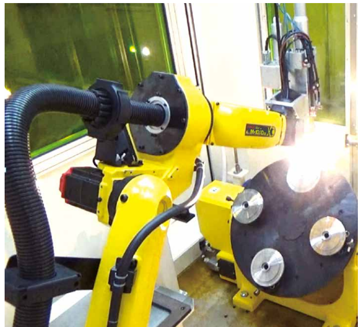
FIBER LASER welding
